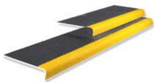
Drill two holes at each end of the Anti-Slip Step Cover, one approximately 15mm in from the back edge and 15mm in from the side. The second hole should be approximately 15mm in from the side and on the line where the black tread meets the yellow or white nosing. It is unlikely that the Anti-Slip Step Covers will require additional fixings in the middle of the tread, (unless the tread is over 2000mm long).
